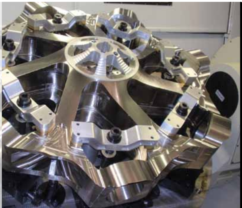
This is the semi-finished 66-inch-diameter main rotor hub mounted in its fixture on the pallet base of the largest of the new five-axis machining centers.
